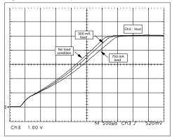
The start up time has also been measured. This is given in figure 13, where both the input and output voltages are given at start up, for a full load condition. The start up time is about 200ms.
