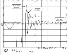
Figure 17. Voltage spikes on auxiliary winding
