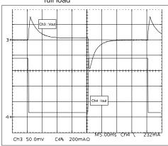
Figure 10. Dynamic behaviour for 7% to 100% of full load
